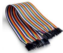
Jumper Wires are used to connect components to each other on the breadboard, and to the Arduino.
